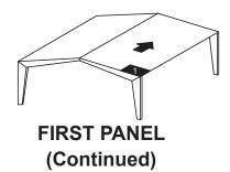
Attach the panel to the eave strut and metal inside closures with 1EFASTENER. Eight fasteners are required at this location.
