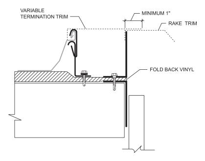
After laying the last insulation run, install the rake support over the insulation along the steel line. Lay the last panel run. Temporarily fasten the male leg to the rake support with vise grips.
