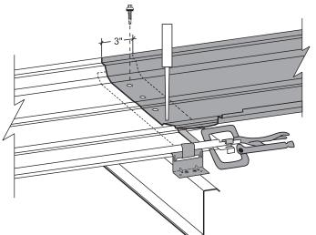
Remove awl and insert in the middle hole nearest the male leg. Install 1EFASTENER in the hole by the female leg.
