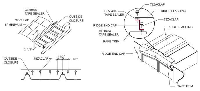
If you do not have a peak box, install a ridge end cap for each end of the ridge flashing.
