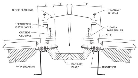
Install the ridge flashing starting and ending 2" outside the steel line. Fasten the ridge flashing to the outside closures with 78ZACLAP. Install a fastener 1" from panel seam on both sides of panel. Install additional fasteners directly above minor ribs of panel. Four fasteners are required at each panel. Leave 6" unfastened on each end to allow for the rake trim to be installed later. DO NOT FASTEN THROUGH THE LOCK OF THE STANDING SEAM.
