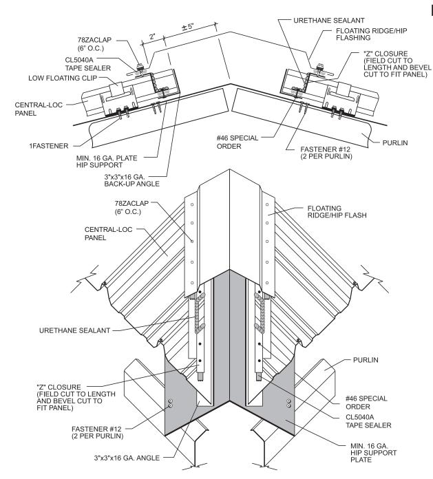
All trapezoidal panels are extremely difficult to install at hips and valleys in a weathertight manner. The use of these details should only be attempted by installation crews that are highly experienced.
