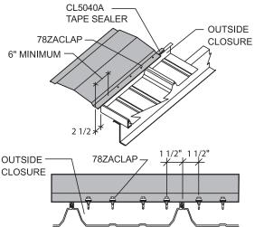
Install the ridge flashing starting and ending 2 1/2" outside the steel line. Fasten the ridge flashing to the outside closures with 78ZACLAP. Install a fastener 1 1/2" from panel seam on both sides of panel. Install additional fasteners directly above minor ribs of panel. Four fasteners are required at each panel. Leave 6" unfastened on each end to allow for the rake trim to be installed later. DO NOT FASTEN THROUGH THE LOCK OF THE STANDING SEAM.
