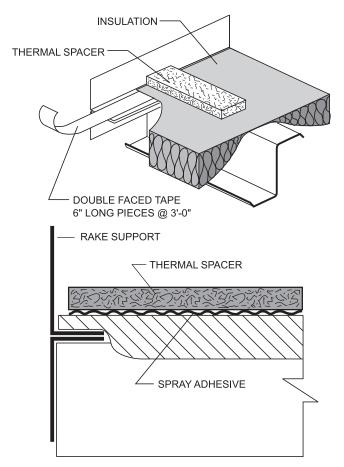
Using spray adhesive, (not by CSMI) adhere the thermal spacer to the insulation. The thermal spacer increases the insulation capacity along the purlins.
