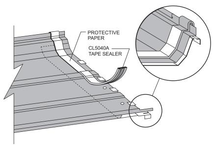
Install CL5040A tape sealer over prepunched holes. Be sure to place the tape sealer over the male leg. DO NOT REMOVE THE PROTECTIVE PAPER AT THIS TIME, EXCEPT AT THE MALE LEG.
