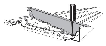
protective paper from tape sealer. Apply tape sealer to the ridge panel just installed. Be sure to seal to the mastic on the previous panel.
