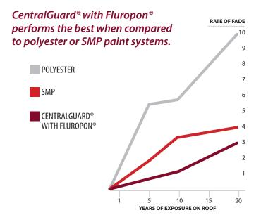
Fade is measured in Hunter units. One Hunter unit denotes the smallest degree of color change visible to the naked eye. Lower numbers are better and mean less fading. Notice how CentralGuard with Fluropon fades much less than other paint systems and at a slower rate over time.
