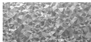
† Weathering and appearance variation, including color, sheen, and spangle, is common in non-painted materials and is not a cause for rejection. For consistent appearance, choose a paint-finished product. Colors on this chart are close representations of actual metal color, limited by printing and viewing conditions. Color matching optimized for outdoor viewing.
